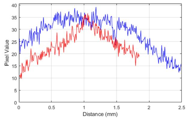
**FIG. 1.** Example pre-explosion image of the high-magnification configuration, with perpendicular lineouts demonstrating the non-uniform intensity profile. Horizontal lineout is left to right, and vertical is top to bottom. The lineouts are averaged over the width of the lines on the radiograph (5 pixels).
