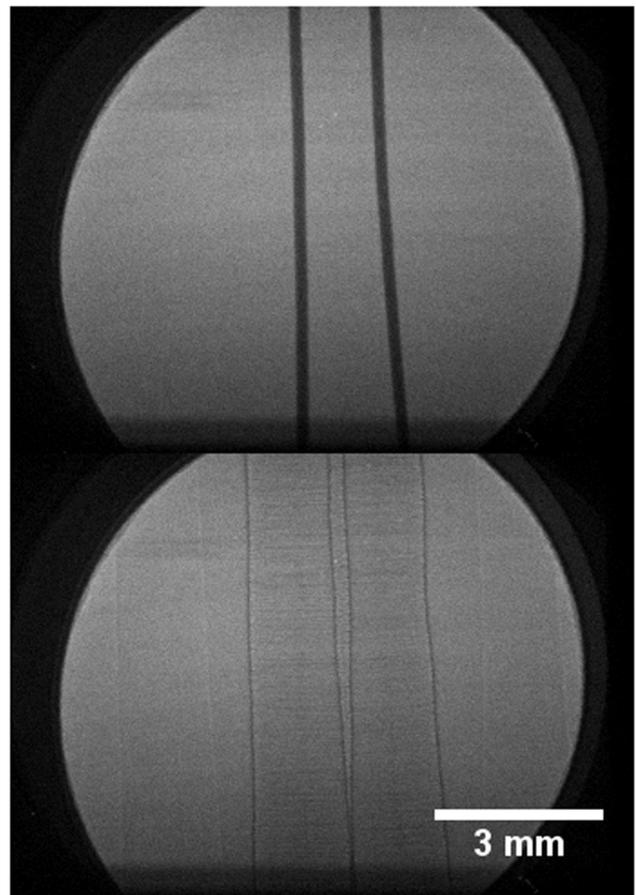
**FIG. 6.** X-ray radiographs of pre- and post-explosion of two parallel  $160 \mu\text{m}$  copper wires in the low magnification configuration. The delay between the two images is 2112 ns (3 frames), with explosion beginning within the first 704 ns.
