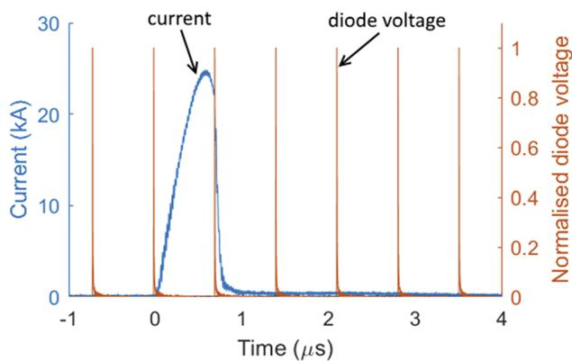
**FIG. 3.** Graph showing the response of the x-ray diode (i.e., timing of the x-ray pulses) and the measured current in the pulser for a single experiment, after correction for cable delays and offset on the x-axis such that the foot of the current pulse is at  $t = 0$ .
