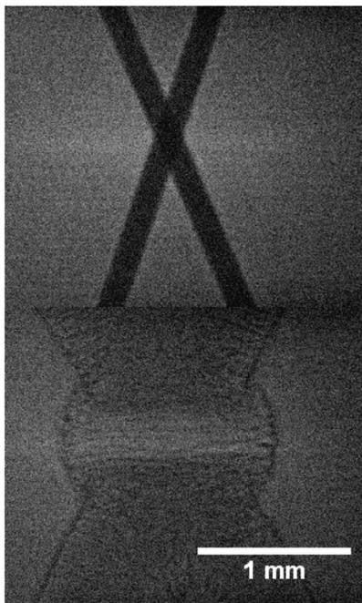
**FIG. 5.** X-ray radiographs of pre- and post-explosion of an x-pinch made using  $160 \mu\text{m}$  copper wires in the high magnification configuration. The delay between the two images is 1408 ns (2 frames), with explosion beginning within the first 704 ns.
