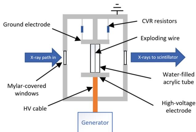
FIG. 2. Cross section diagram of experimental chamber.
