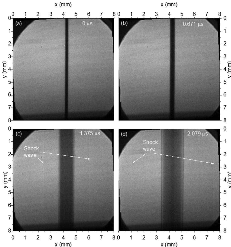
FIG. 4. Typical low-resolution images of an exploding tungsten wire.
