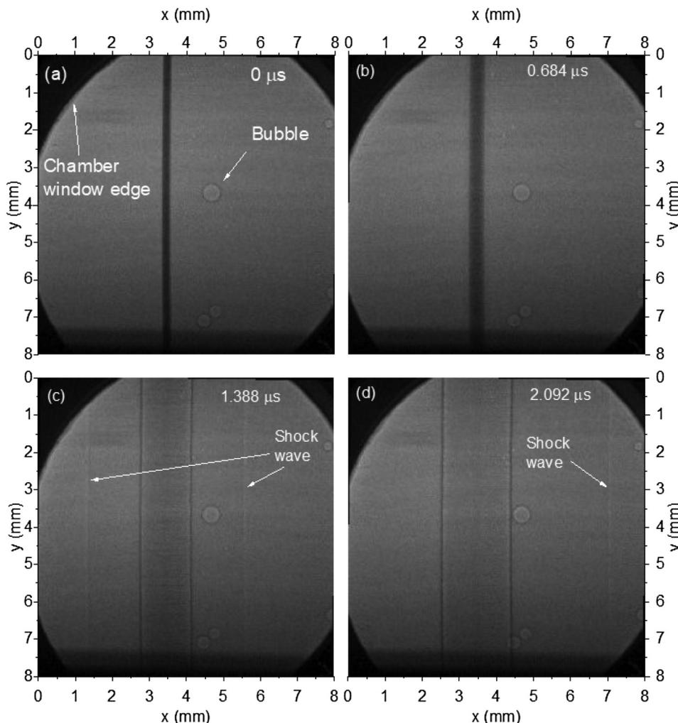
FIG. 3. Typical low-resolution images of an exploding copper wire.
