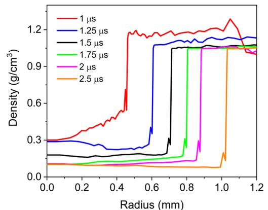
FIG. 10. Radial density distribution of an exploding copper wire obtained by MHD simulation (The plateaus to the right,  $\sim 1 \text{ g}/\text{cm}^3$ , are water surrounding the wire).
