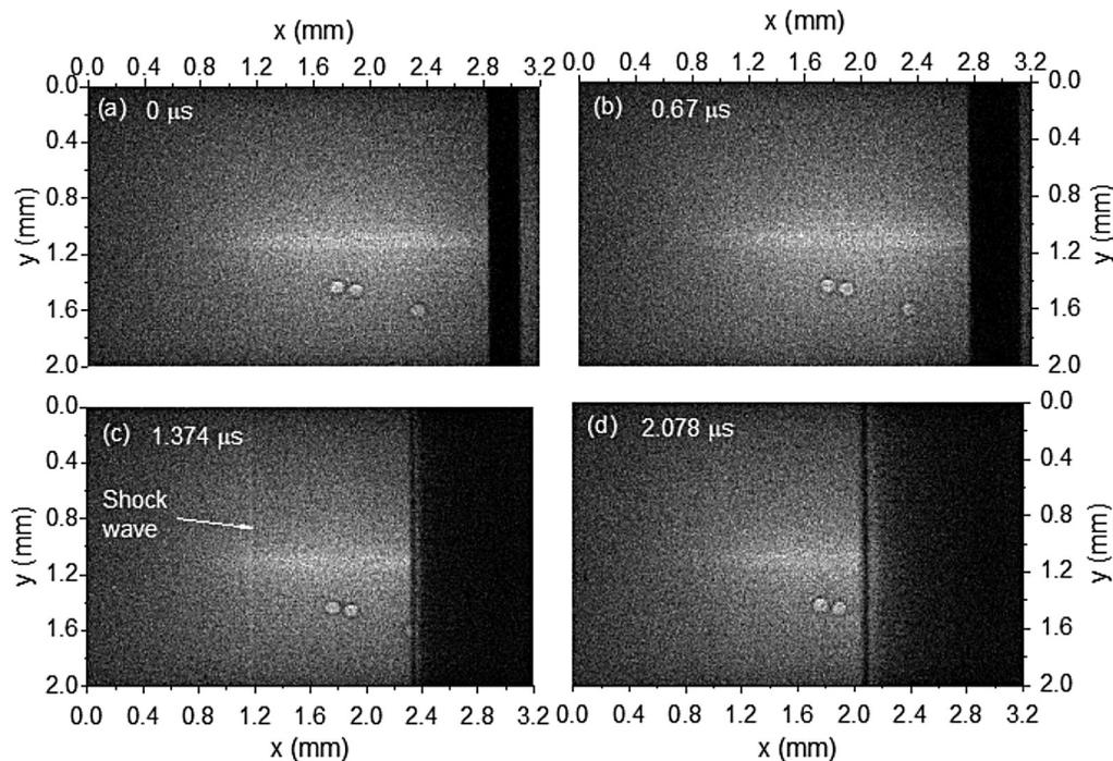
FIG. 6. Typical high-resolution images of an exploding tungsten wire.
