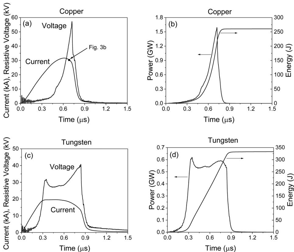
FIG. 2. Measured current and resistive voltage, and calculated power and energy input waveforms for copper [(a) and (b)] and tungsten [(c) and (d)] wires. [The marker in (a) is to clarify where the image in Fig. 3(b) is in time.]
