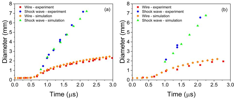
FIG. 7. Comparison between experimental and simulation diameters of the wire and position of the shock wave for (a) copper and (b) tungsten.
