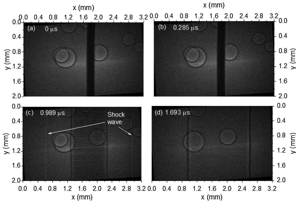
FIG. 5. Typical high-resolution images of an exploding copper wire.
