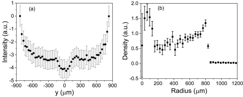
FIG. 9. (a) Absorption profile of the exploding copper wire at  $2.092\mu\text{s}$  delay from the beginning of the rise of the current, and (b) the Abel transform of this absorption profile.
