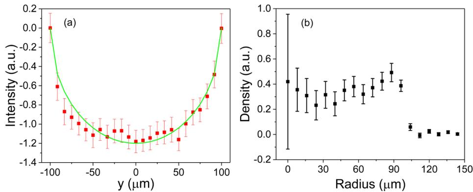
FIG. 11. (a) Absorption profile of a copper wire before explosion along with the theoretical curve. (b) Inverse Abel transform of the wire before explosion.
