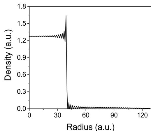
FIG. 8. Reconstruction of a perfect wire with uniform density using Abel inversion.
