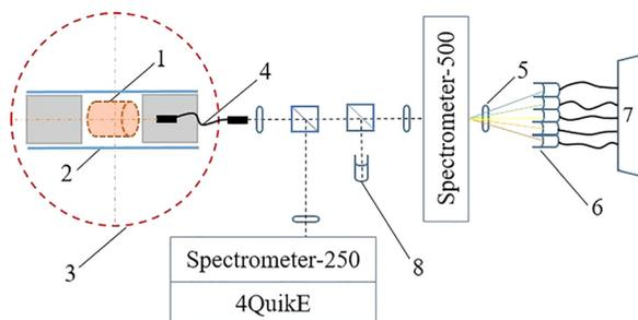
FIG. 2. Optical diagnostic scheme. 1—plasma; 2—capillary; 3—spherical wire array; 4—optical fiber; 5—cylindrical lens; 6—fiber bundle array; 7—9-channel PMT array; and 8—single PMT.
