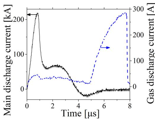
FIG. 1. Typical waveforms of the main discharge current (solid line) and the current between the two electrodes placed inside the capillary (dashed line).
