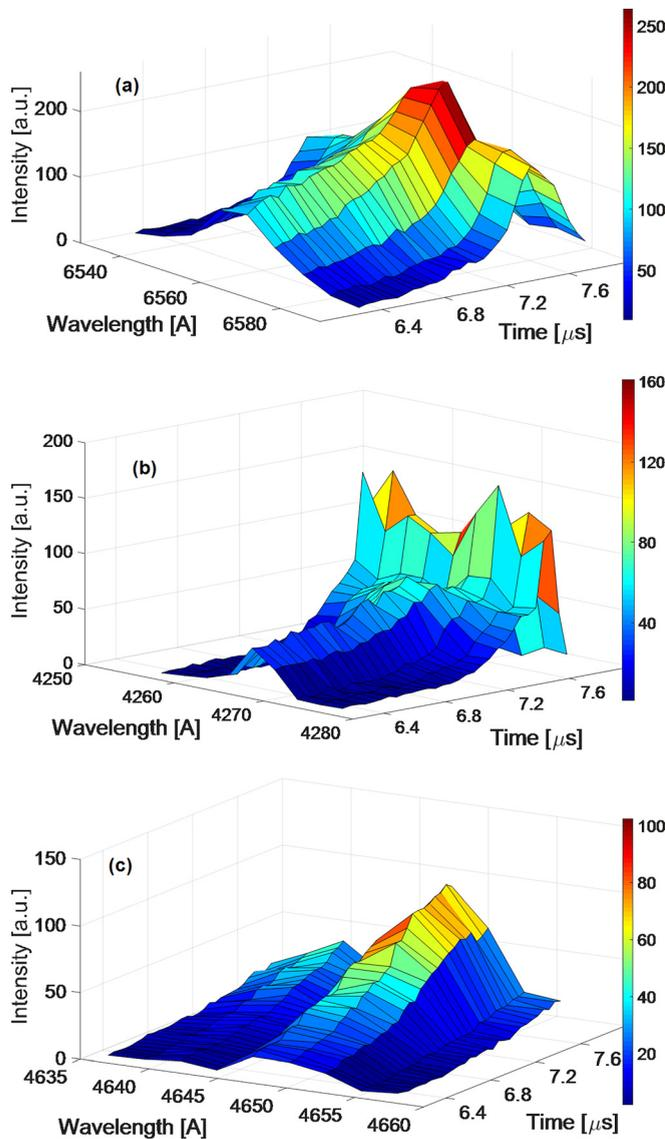
FIG. 3. Time evolution of  $H_\alpha$  (a), C II (b), and C III (c) spectral lines.
