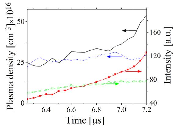
FIG. 4. Time-dependent evolution of the  $H_\alpha$  spectral line intensity and plasma electron density without (dashed lines) and with wire array explosion (solid lines).
