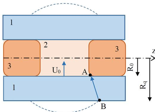
FIG. 7. A schematic model of the plasma compression in the capillary. 1—capillary; 2—plasma; 3—electrodes;  $R_0$  and  $R_q$ —inner and outer capillary radii, respectively;  $U_0$ —the velocity of the inner capillary wall; dashed line—front of a spherical SSW in water.
