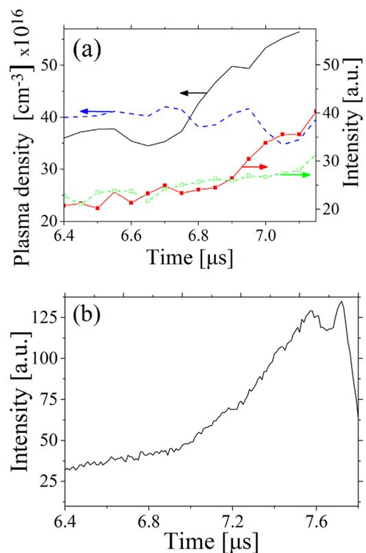
FIG. 5. Temporal evolution of (a) the C II (4267 Å) line intensity and plasma electron density without (dashed lines) and with wire array explosion (solid lines); (b) total light emission registered by a single PMT.
