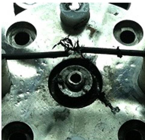
FIG. 4. Equatorially placed fiber after the experiment with explosion of 30 mm in diameter Cu wire array.
