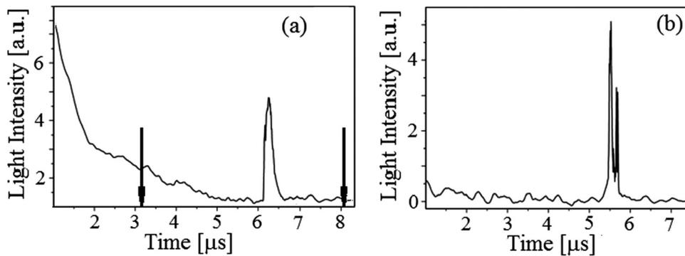
FIG. 3. Typical waveform of the (a) water and (b) fiber light emission. Explosion of Cu wire array. Arrows corresponds to the appearance of water light emission in the case of 20-mm- and 40-mm-diameter Cu wire array explosion.
