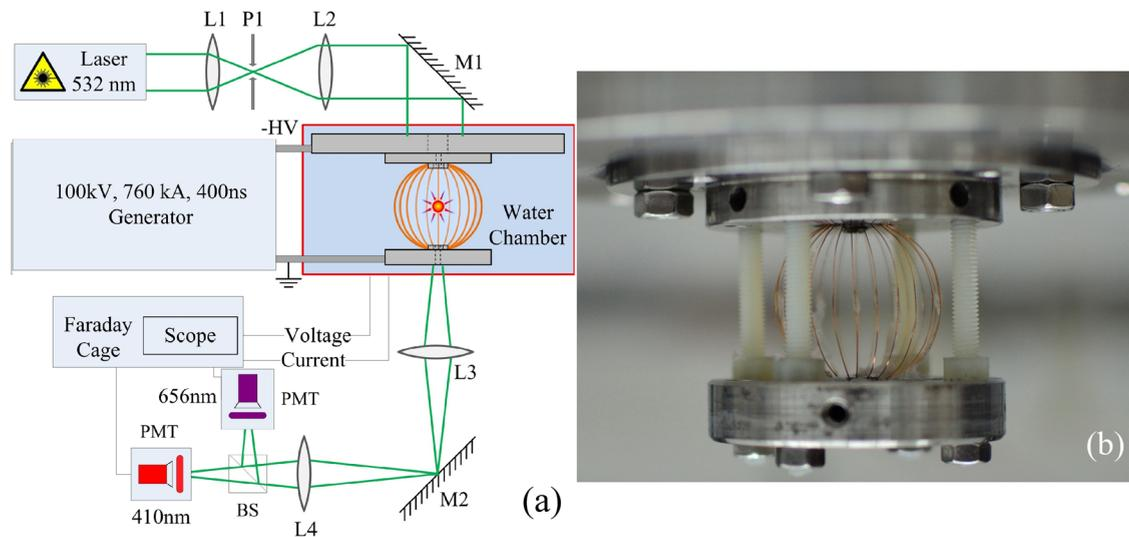
FIG. 1. (a). Experimental setup. (b) External view of 40 Cu wires array of 30 mm in diameter; each wire is of 114  $\mu\text{m}$  in diameter.
