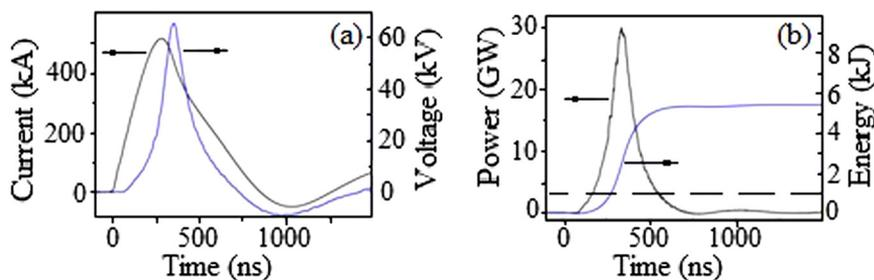
FIG. 2. Waveforms of (a) the current, resistive voltage, and (b) power and energy. 30 mm in diameter spherical Cu wire array; 40 wires each of 114  $\mu\text{m}$  in diameter. Dotted line in (b) is the energy required for complete evaporation of Cu wires.
