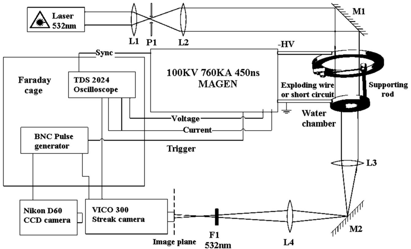
FIG. 1. Experimental setup.
