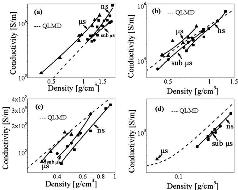
FIG. 7. Comparison between conductivity values of Al for different timescales at temperatures of (a) 10 KK, (b) 20 KK, (c) 30 KK, and (d) 40 KK. Symbols denote experimental results, solid lines denote interpolated fitting of those results, and dashed lines denote QLMD model.
