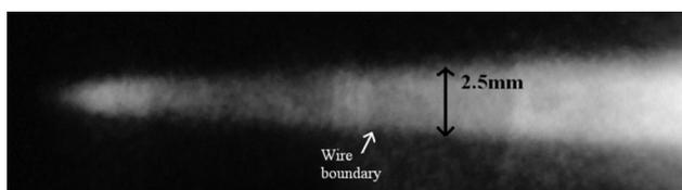
FIG. 2. Streak image of exploding 0.38 mm diameter Al wire (no backlighting).
