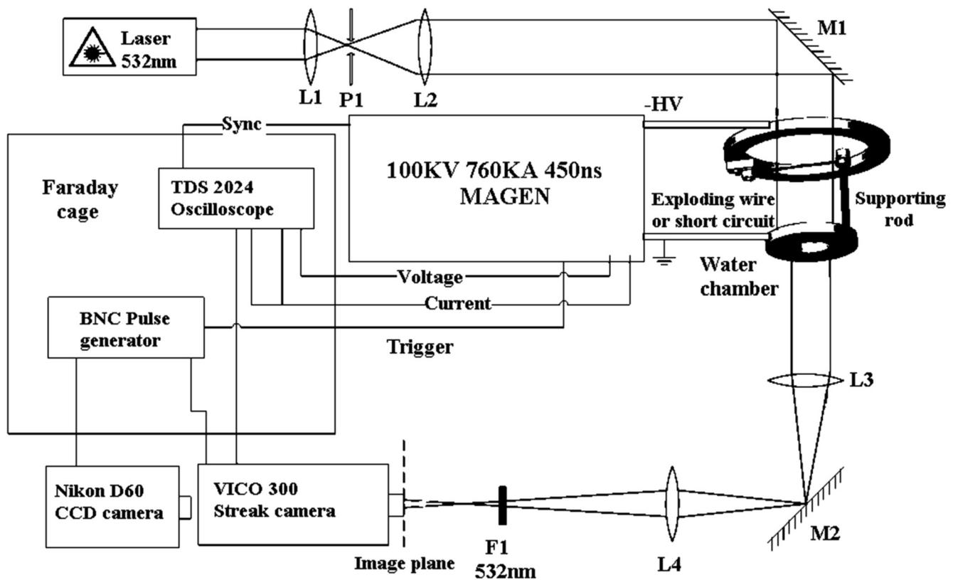
FIG. 1. Experimental setup.
