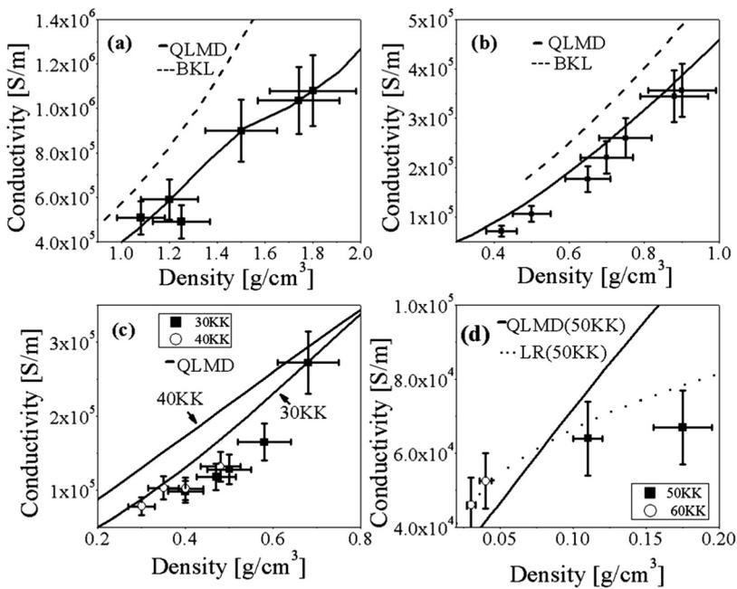
FIG. 6. Electrical conductivity of Al for temperatures of (a) 10 KK, (b) 20 KK, (c) 30–40 KK, and (d) 50–60 KK. Symbols denote experimental results, the solid line denotes QLMD model, the dashed line denotes BKL model, and the dotted line denotes LR model.
