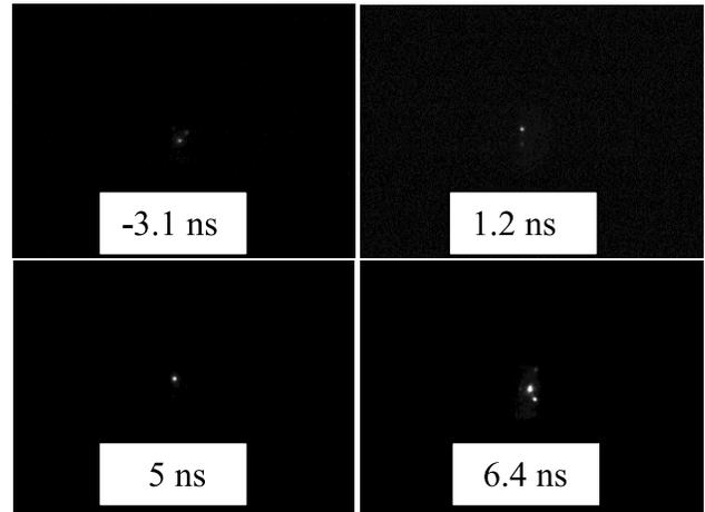
Fig. 4. Top-view images recorded at  $2 \times 10^5$ -Pa pressure with 4QuikE camera with 3-ns exposure time at different time shifts  $\Delta_{c-\mu w}$ .
