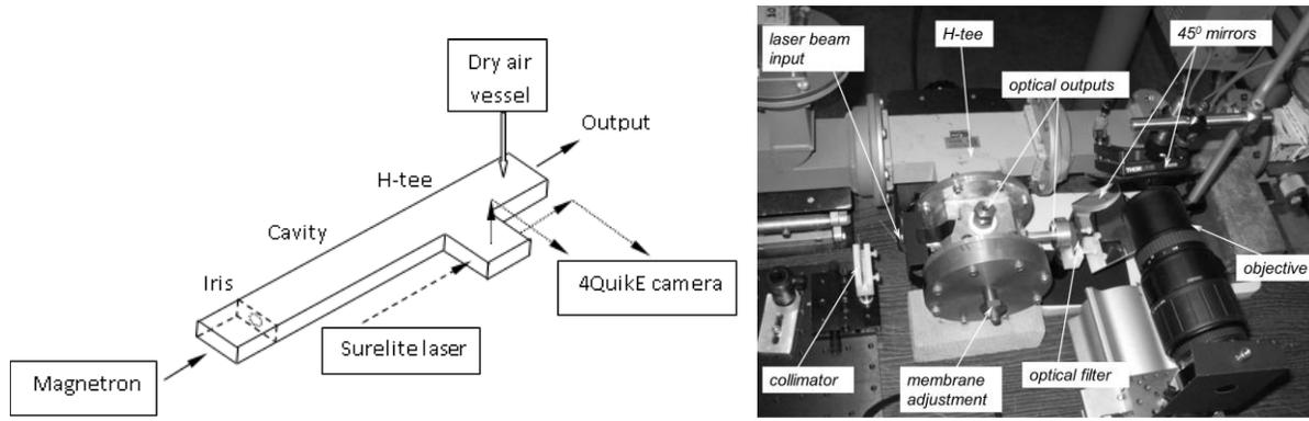
Fig. 1. Left: schematic of the experimental setup. Right: setup for fast-framing imaging of the microwave plasma discharge.
