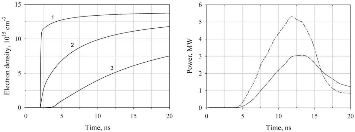
Fig. 7. MAGIC simulation of the energy release from the compressor cavity in the gas conductivity model for air at  $2 \times 10^5$ -Pa pressure for  $Q_0 = 2 \times 10^{26} \text{ cm}^{-3} \cdot \text{s}^{-1}$ . Left: electron density within the plasma filament versus time at  $z =$ : 1–0.5 mm; 2–3.5 mm; 3–12.5 mm. Right: microwave power at the output port versus time (dashed curve is for the case  $Q_0 = 10^{27} \text{ cm}^{-3} \cdot \text{s}^{-1}$ ).
