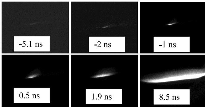
Fig. 3. Side-view images recorded at  $2 \times 10^5$ -Pa pressure with 4QuikE camera at different time shifts  $\Delta_{c-\mu w}$ . The exposure time is 2 ns; the camera gain is close to maximal one. The input power is of  $\sim 310$  kW.
