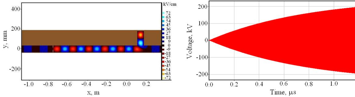
Fig. 6. Results of the MAGIC simulation of the compressor charging used to preset initial fields in simulations of microwave extraction. Left: contour plot of the  $E_z$ -field in the  $x$ - $y$  plane. Right: build-up of the RF voltage across the waveguide in the field antinode in the middle of the cavity (between the input iris and tee side arm). The voltage amplitude of the wave entering the system in the  $TE_{10}$  mode is 15 kV.
