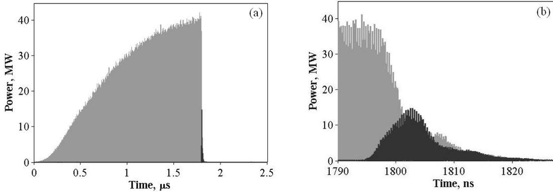
Fig. 2. (a) Instantaneous power of the output (dark gray) and cavity signals recorded when the maximal output power was achieved. (b) Same as (a) in the ns timescale.
