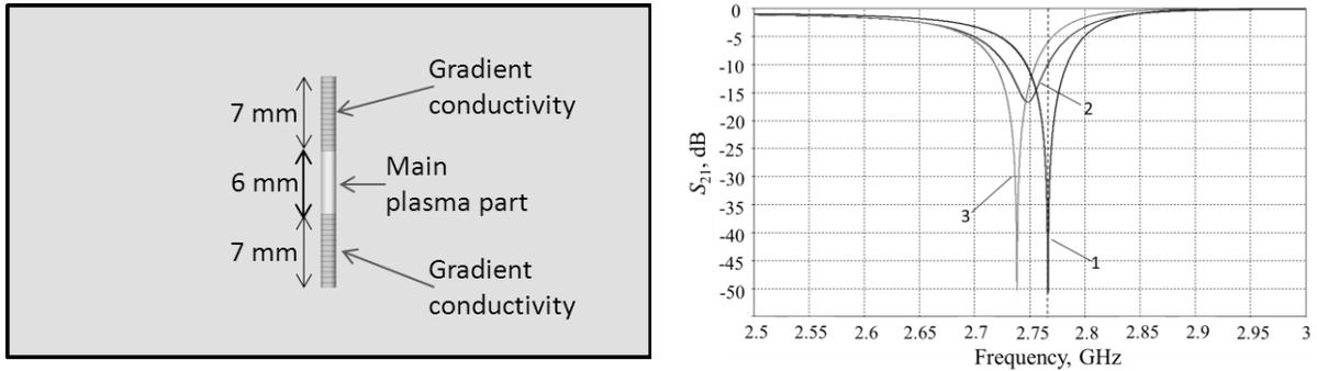
Fig. 5. Left: configuration of the conductive gas (plasma) filament in the WR284 waveguide cross section taken for CST simulations. Right: frequency response of the H-plane tee with the conductive gas filament in the shorted side arm. The conductivity in the main part  $\sigma_0 = 1-0$ ;  $2-2.3 \times 10^3 \Omega^{-1}\text{m}^{-1}$ ;  $3-2.7 \times 10^7 \Omega^{-1}\text{m}^{-1}$ . The vertical dashed line shows the closing frequency of the tee in the absence of plasma.
