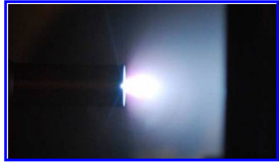
Fig. 7 HTHC (SHC-M1) running in diode mode. The discharge current is 0.9 A, the Xe-gas flow is 1.5 sccm, and the orifice plate–anode gap is 2 cm.
