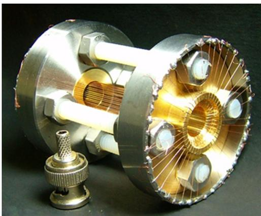
FIG. 1. External view of a cylindrical wire array consisting of 40 Cu wires, each 40 mm in length and  $100 \mu\text{m}$  in diameter.
