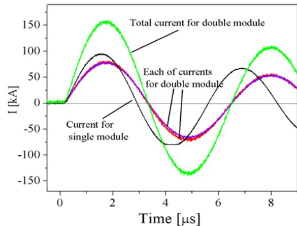
**Fig. 5 Short circuit current wave forms.**
