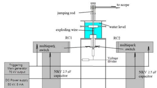
**Fig. 2** Experimental setup for two generators operating on joint load. RC1 and RC2 are Rogowski coils.
