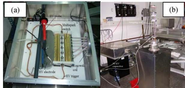
**Fig. 1** External view of the experimental setup: (a) Block of the multi-spark switch with the removed cover; (b) experimental setup with one pulsed generator.
