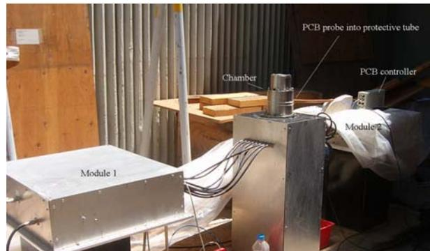
**Fig. 3** Double module setup outside of the laboratory hall for experiments with underwater electrical wire explosion.
