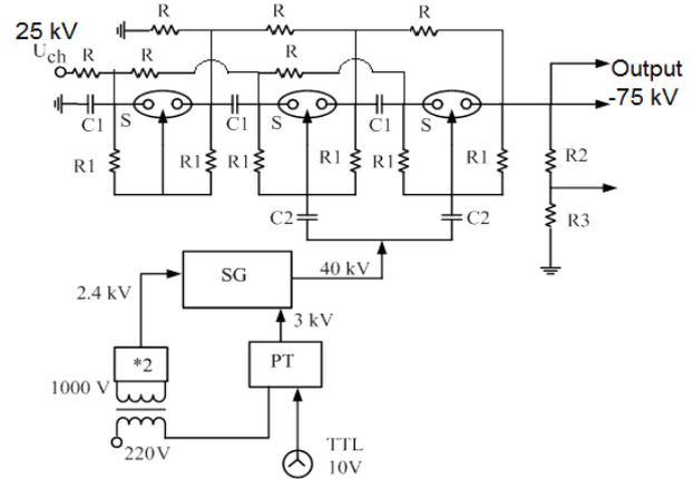
**Fig. 4 High-voltage trigger generator scheme.** C—40 nF, 50 kV Maxwell capacitors; C2—130 pF 40 kV capacitors, S—spark gap switches, Resistance R1 = 200 M $\Omega$ , R2 and R3 are resistances of the voltage divider: R2 = 50  $\Omega$ , R3 = 1  $\Omega$ , SG—spiral generator, PT—pulse transformer, #2—voltage multiplier and rectifier. R = 10 k $\Omega$ —charging resistors.
