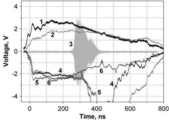
Fig. 11. Accelerating voltage (1, 200 kV/div.), diode current (2, 5 kA/div.), and RF voltage (3) along with the signals from the collimated FCs placed 1 cm behind the vircator cavity at: 4–5 mm off axis; 5–17 mm off axis; 6–30 mm off axis.  $d_{AK} = 20$  mm,  $U_{ch} = 32$  kV.
