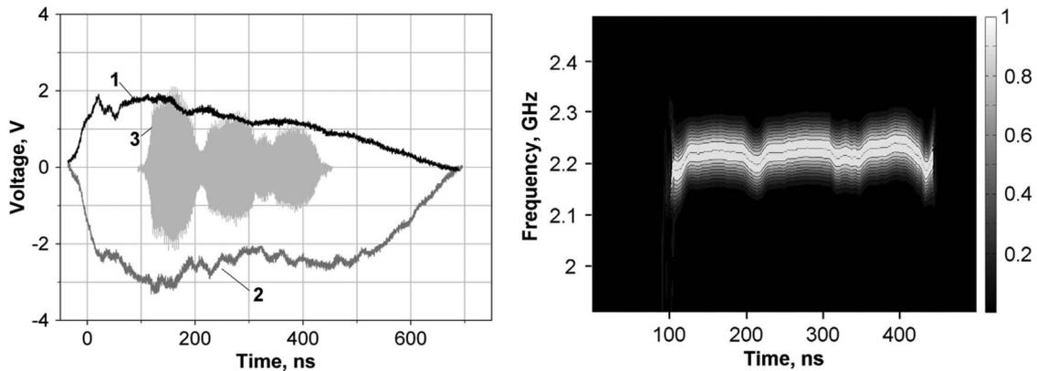
Fig. 5. Left: Accelerating voltage (1, 200 kV/div.), diode current measured by the RC (2, 5 kA/div.), and RF voltage from the B-dot probe (3). Right: Time variation of the radiation spectrum (the RF voltage Fourier transform within the 30-ns time window being shifted by a 1-ns time step). Cathode of [16],  $d_{AK} = 19$  mm, cavity geometry of [16].
