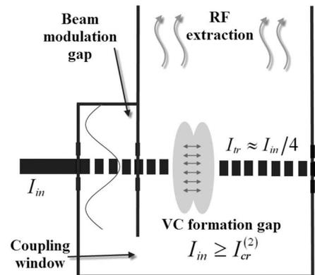
Fig. 1. Schematic of the double-gap vircator interaction space.
