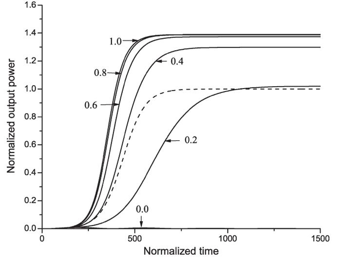
Fig. 3. Dependence of the normalized power on time. “Short” delay time  $\theta < Q_{leak}/|q|$ . Dashed line corresponds to  $q = 0$ . The curves are marked by corresponding  $\alpha/\pi$  values.  $|Q_{diss}| = 15$ ,  $Q_{leak} = 20$ ,  $q = 0.2$ , and  $\theta = 70$ .
